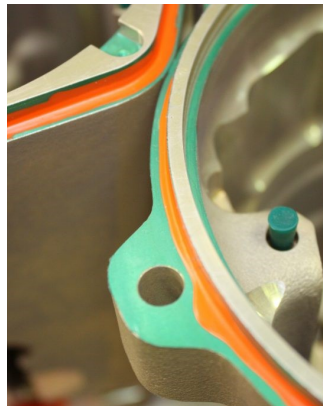
An aluminum part ready for anodizing with masking and plugged holes.
